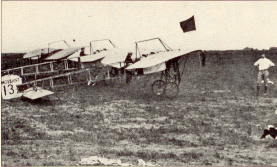
Three Moisant 30-hp monoplanes line up for students' first flights. This "supervised solo" method used airplanes of limited speed and altitude.
